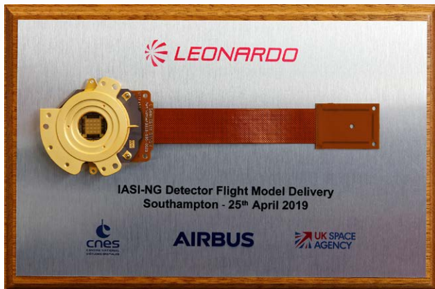
Photo: Egide metallic and ceramic package protecting Leonardo's detector
